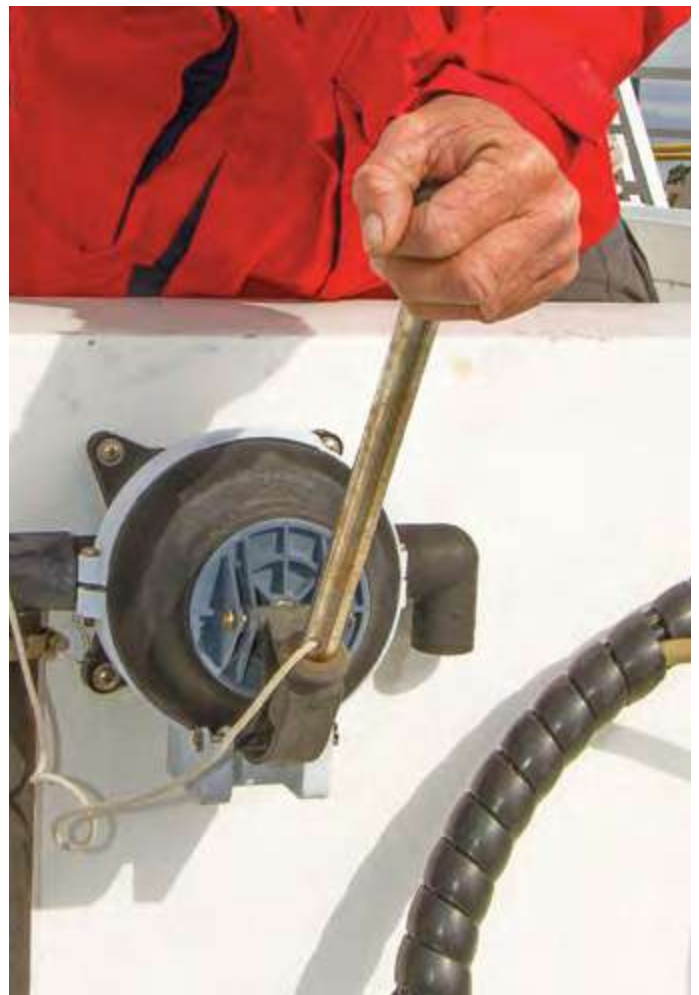
A bilge pump can be manually, electrically or mechanically operated
