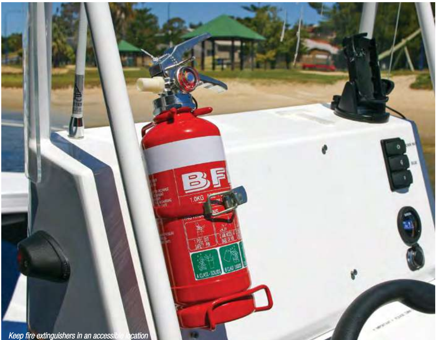
Check the gauge is in the green
